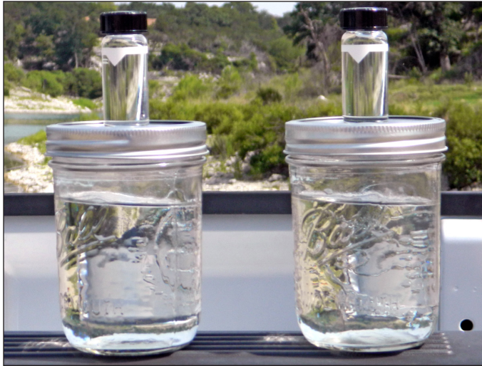
The effluent sample on the left, discharged from the Orenco AX100 unit, is almost indistinguishable from a water sample taken directly from Lake Belton. Weekly effluent tests from the AX system show consistently better results than are required by the TCEQ.
