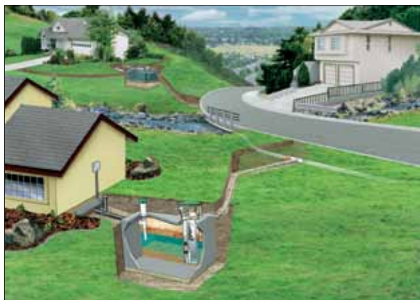
Effluent sewers are an affordable, phase-able sewer option that doesn't burden current residents with high rates for future system growth.
