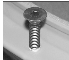
Close-up views of stainless steel self-tapping screw in Ultra-Rib riser
